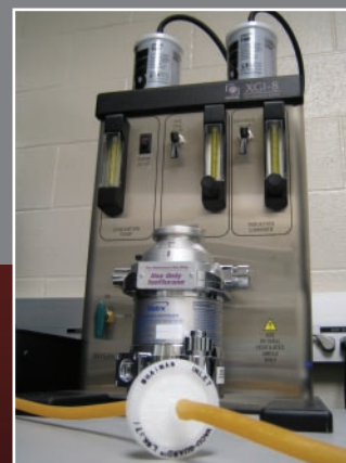
Vacu-Guard® filters, encapsulated in a polypropylene (PP) housing and fully hydrophobic PTFE membrane with a pore size of 0.1um prevents escape of microorganisms. Retention rate is 99.97%, withstanding a maximum pressure of up to 20psi.
